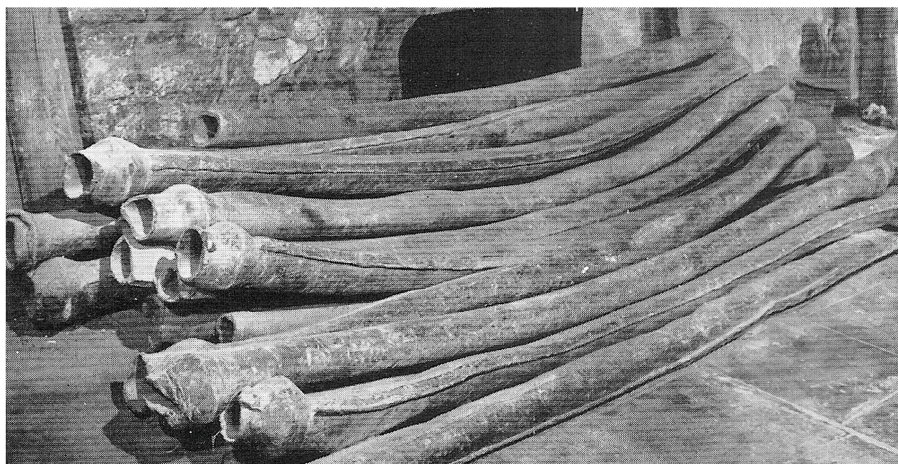
Fig. 10. Lead conduits, 3 m long, retrieved from the Rhône river near Arles, of siphon that crossed the Rhône River (Arles Museum).
